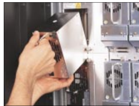
The Neo Series features redundant power supplies that can be replaced without interruption. (Available with 4000 models only.)
