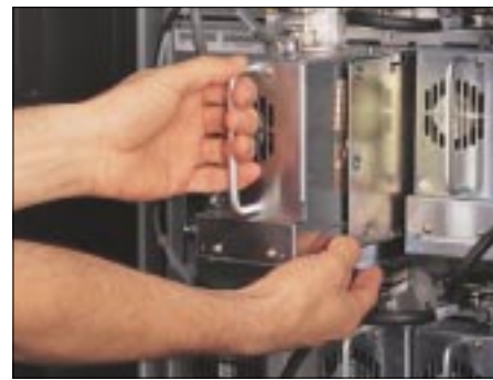
Neo's LiveSwap™ lets you move tape drives without interrupting SCSI bus operations.
